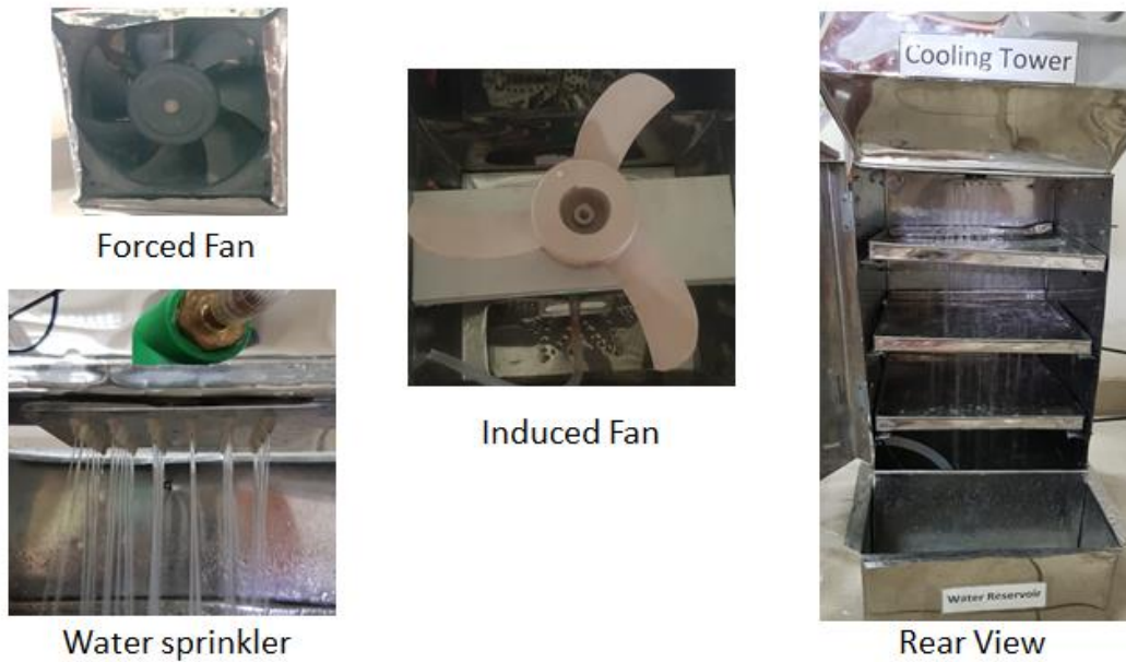
Figure 15: Cooling tower Experiment Arrangement
