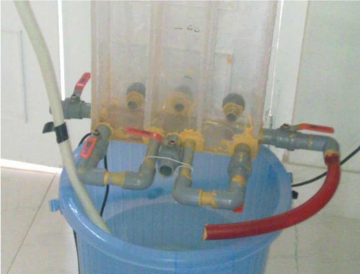
Figure 4.26: Magnified picture of Actual plant (Water level control of Three Tank System)
