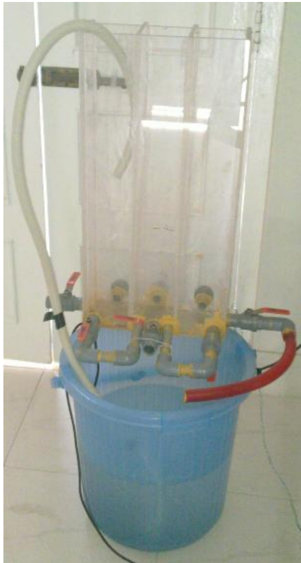
Figure 4.25: Actual plant (Water level control of Three Tank System)
