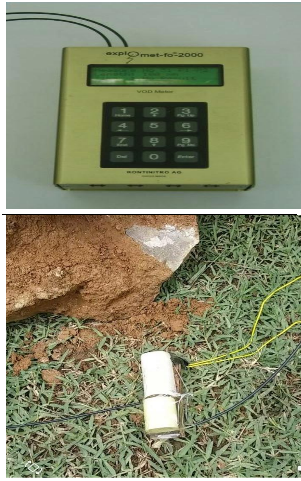
Figure 3.7: Explomet-fo-2000 & Test Sample ready to fire.
