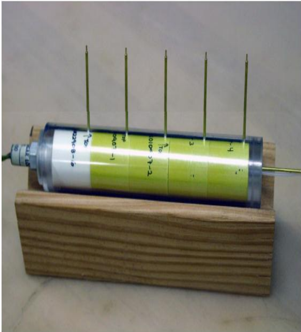
Figure 2.3: Rate stick demonstration cylinder
