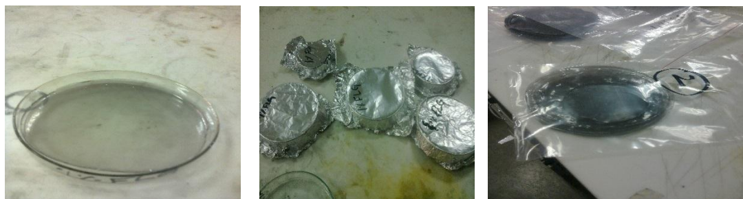
Figure 11: a. Pouring of solution, b. covering with foil, c. dry film
