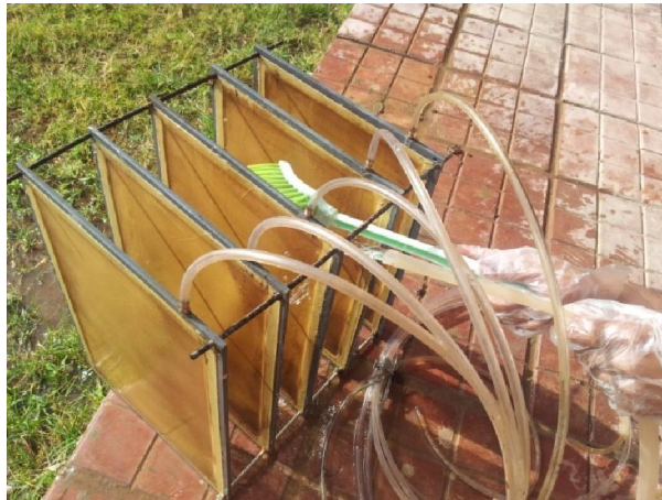
Figure 3.6: Physical cleaning of membrane module with brush
