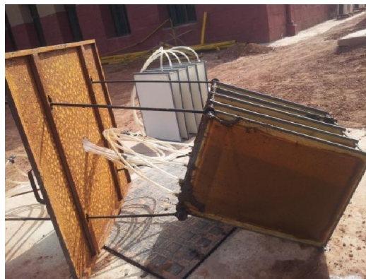
Figure 3.5: Membrane module along with steel rods
