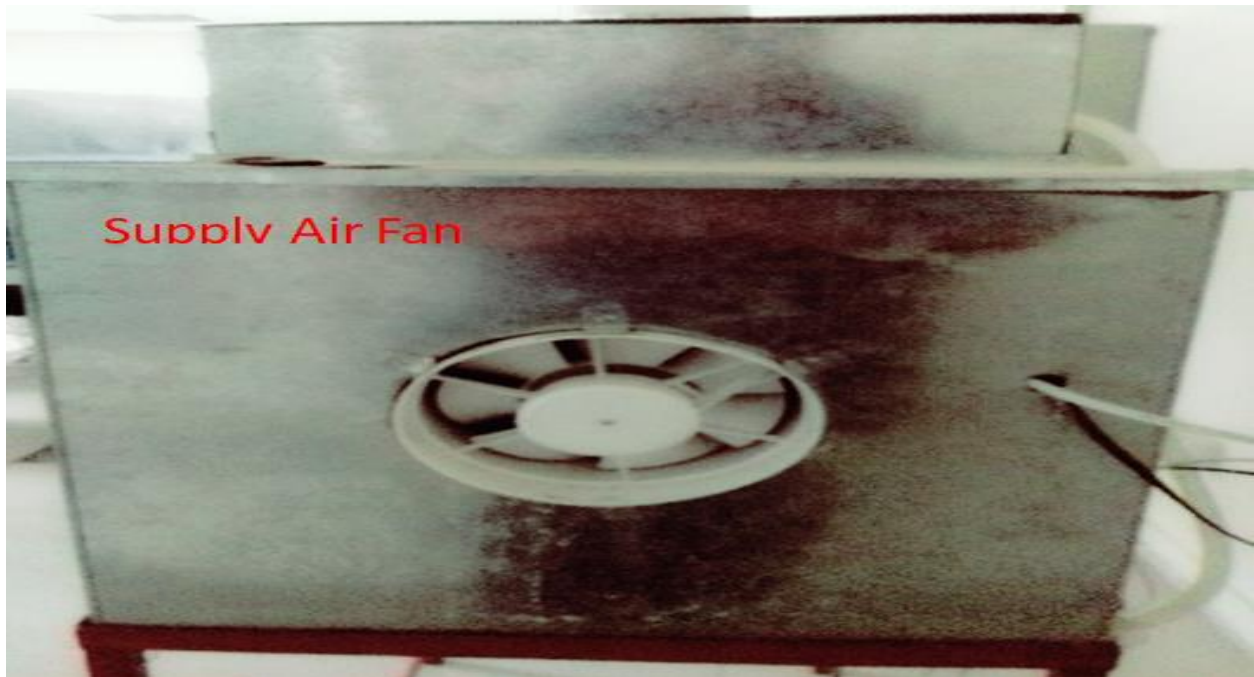
Figure 14: b Inlet Fan.
