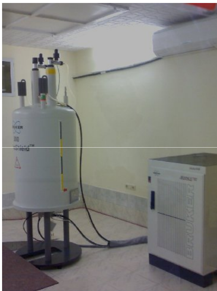
Figure 2.8 Bruker 300 MHz spectrometer, used to obtain NMR spectra.
