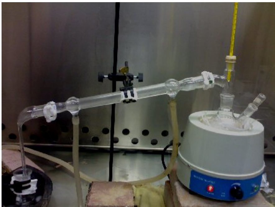
Figure 2.2 Glassware assembly used for the lab preparation of acryloyl chloride.
