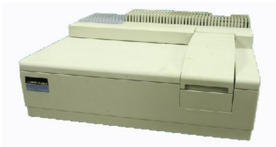
Figure 2.6 Perkin Elmer Lambda 20 spectrophotometer, used to UV-Vis Spectra
