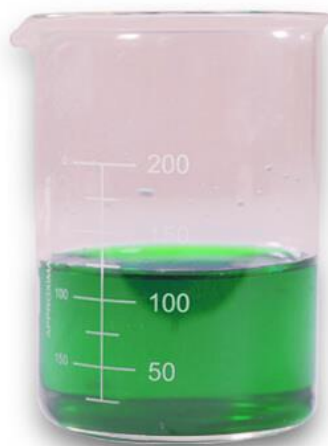
Figure 4.1 As prepared 0.15 M Nickel (II) Nitrate hexahydrate [ \text{Ni}(\text{NO}_3)_2 \cdot 6\text{H}_2\text{O} ] aqueous solution
