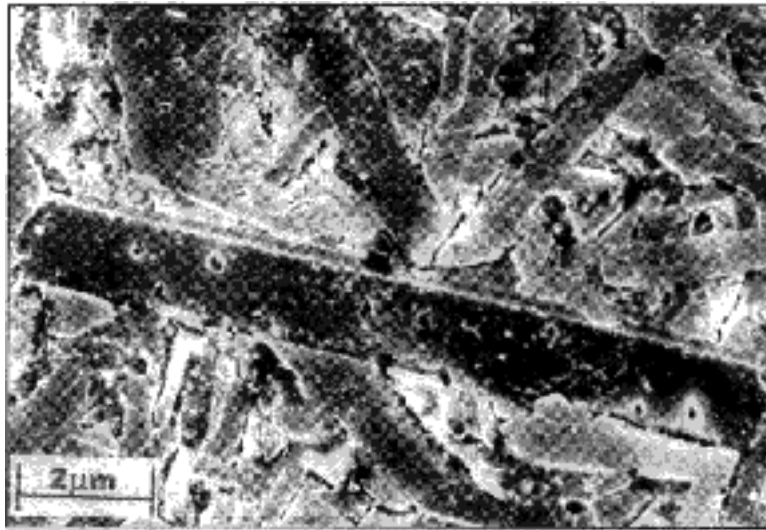
Figure 2.32: TEM photo of \alpha -SiC sintered in argon.
