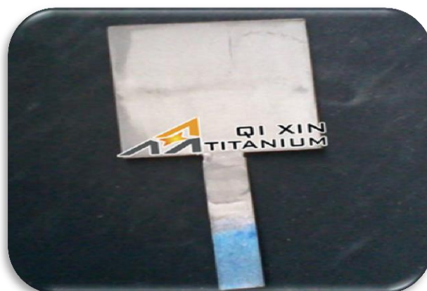
Fig.3.11 Platinum Coated over Titanium Electrode
