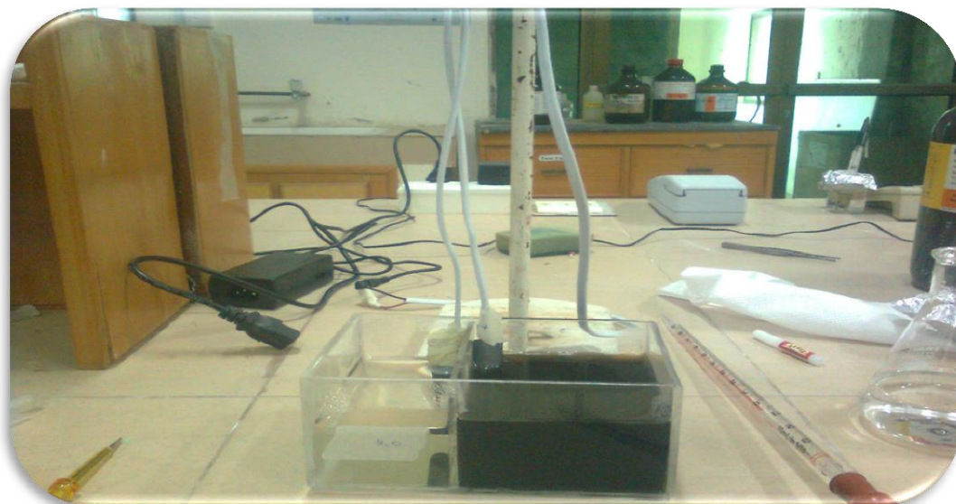
Figure B-5 Carbon Anode Dissociation at 24 V in 1.0 Molar Concentration NaOH Solution
