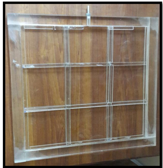
Figure A5: Flat sheet membrane module and Casing
