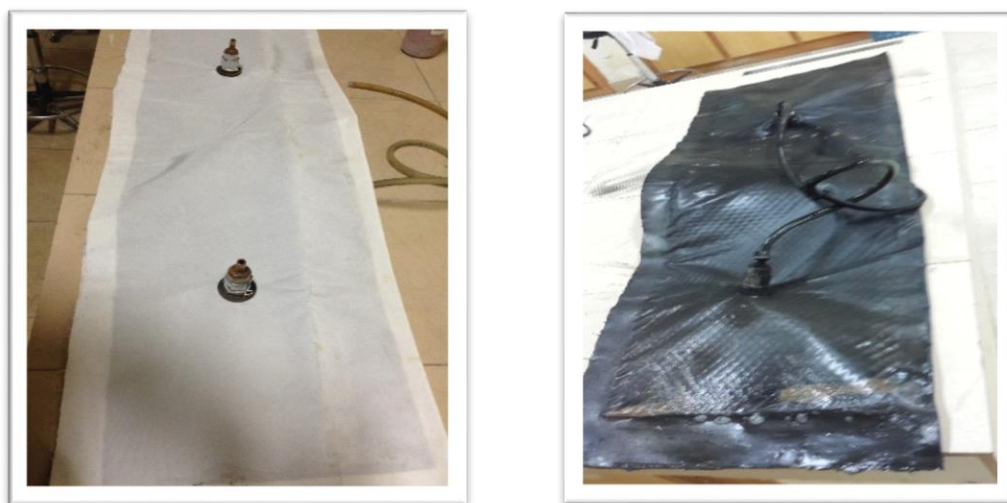
Figure 3.9: Clean membrane and clogged membrane
