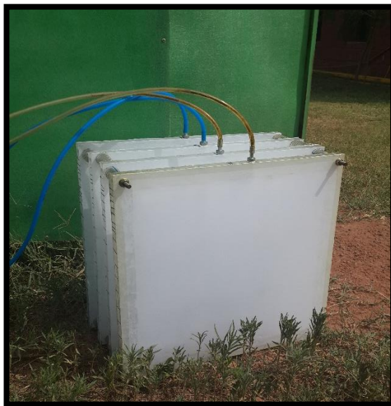
Figure A5: Flat sheet membrane module and Casing
