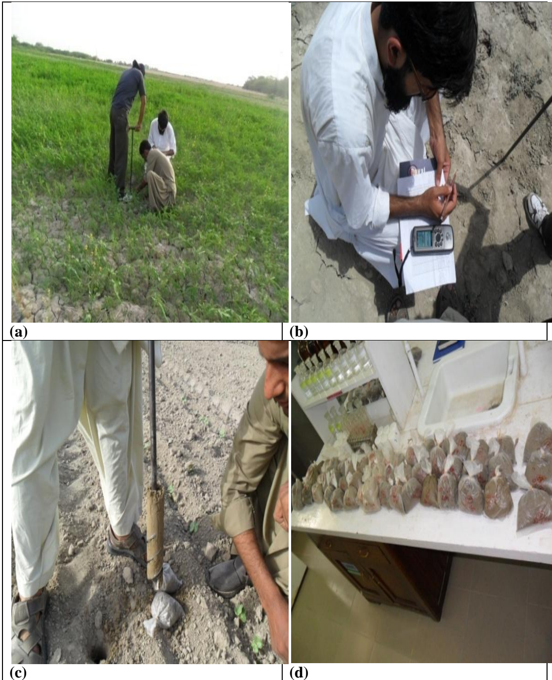
Figure 5. (a) Field sampling carried out by using soil auger (b) GPS points were taken for each sample (c) packing of soil samples in polythene bags (d) samples ready for lab analysis.
