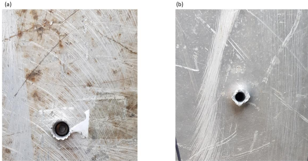
Figure 6.2: Base Armor Plate showing impact of 7.62 x 51 mm AP Hard Core Bullet (a) Impact Side (b) Distal Side
