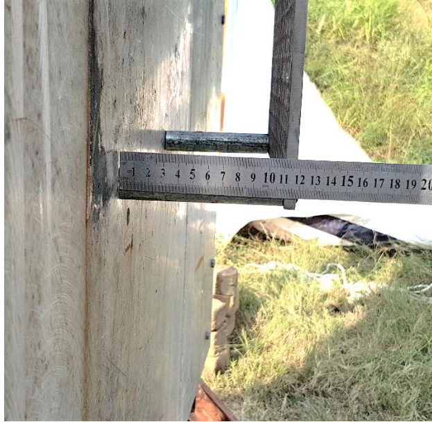
Figure 3.5: High Hardness perforated plated mounted on Aluminum Base Plate Side View
