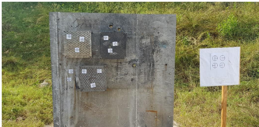
Figure 3.4: High Hardness perforated plated mounted on Aluminum Base Plate
