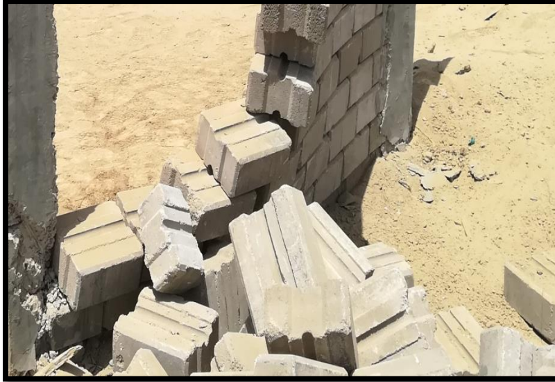
Figure 4. 23 Groves of eco-blocks after test 4
