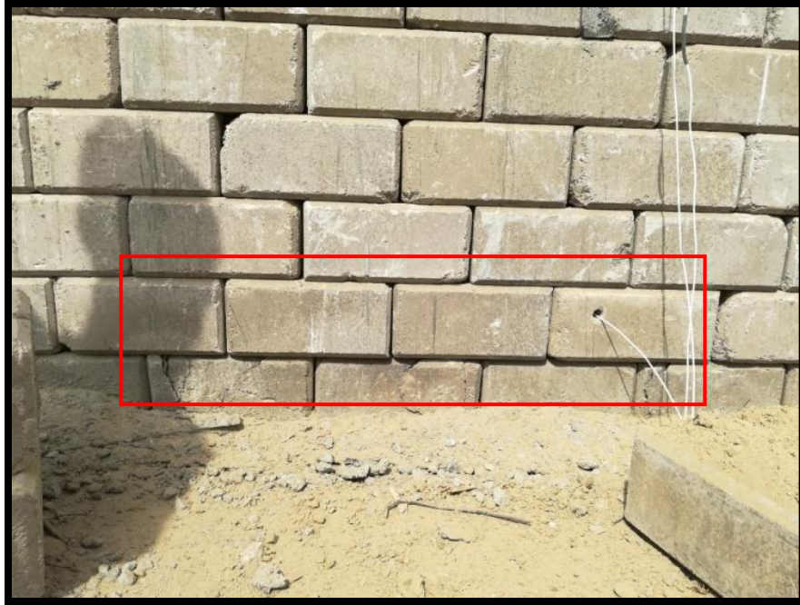
Figure 4. 14 Bulging of wall after blast test
