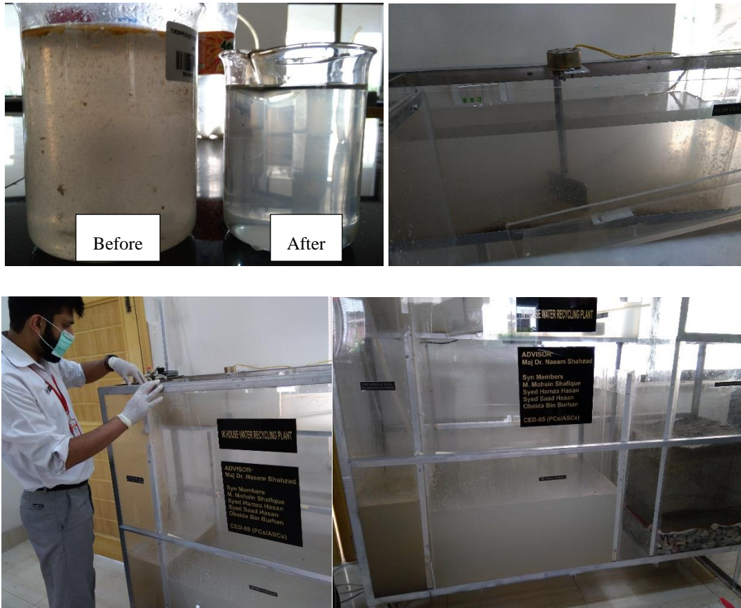
Figure 3.15: Treatment of Greywater and Samples Before & After Treatment
