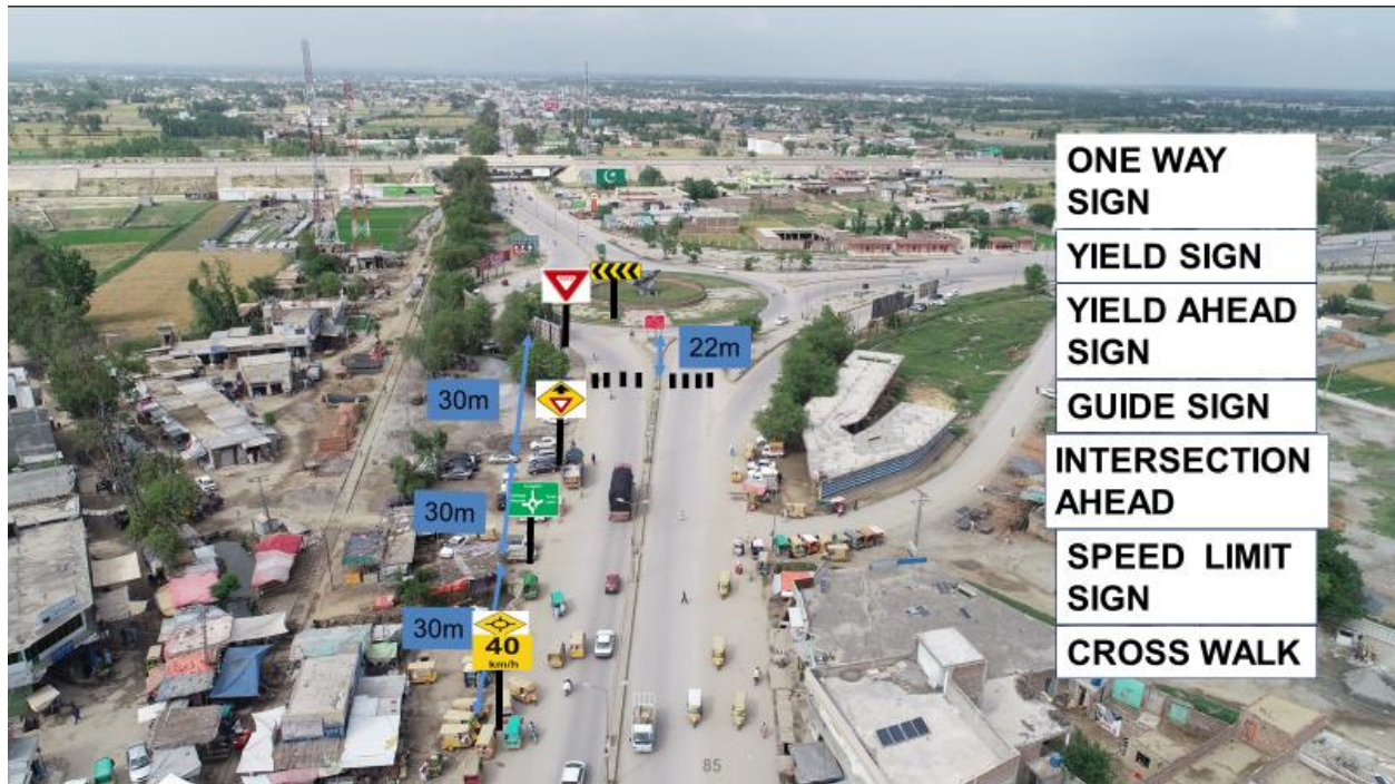
Figure 16 Signage Plan for Rashakai Roundabout South.
