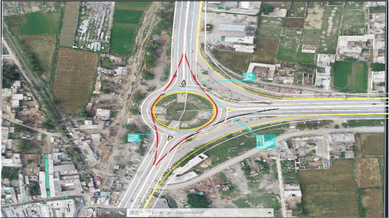
Figure 12 Shows Existing Design of Rashakai Roundabout South
