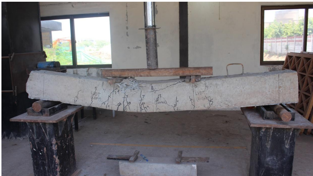
Figure 5-1: Failure of B-1
