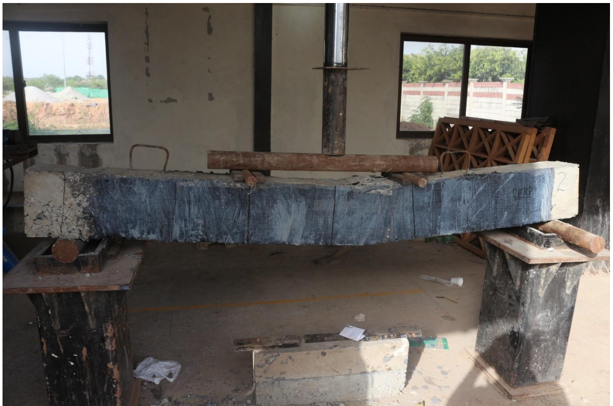
Figure 5-3: Failure of Fully jacketed beam specimen, B2
