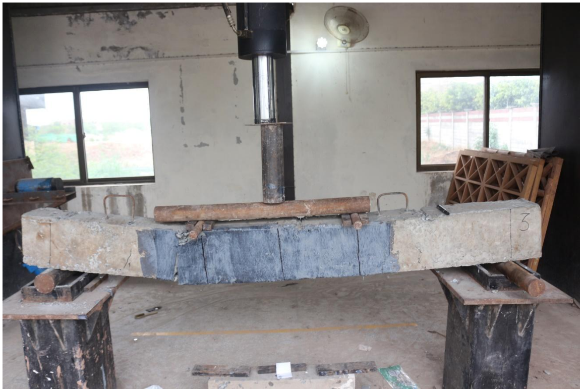
Figure 5-5: Failure of selectively jacketed specimen
