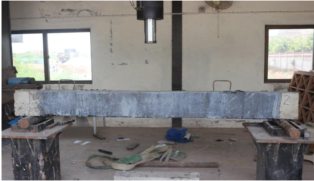
Figure 4-6: Wrapping of a beam specimen with CFRP using Dry Process
