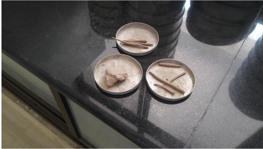
Figure 3.5 Oven Dried Samples of PL and LL
