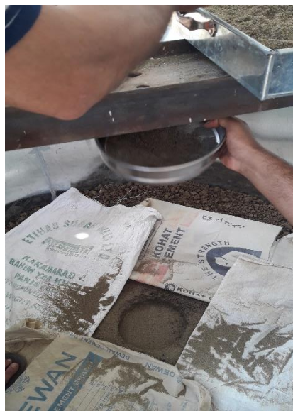
Figure 3.20 Sand replacement with raining compaction
