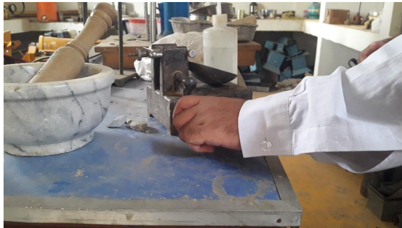
Figure 3.4 Liquid Limit using Casagrande Apparatus
