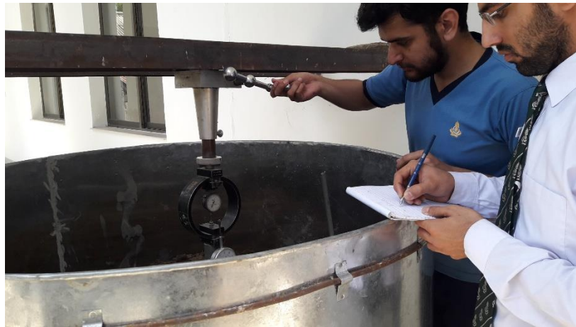
Figure 3.17 CBR load test
