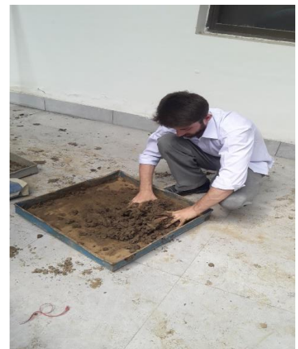
Figure 3.10 Mixing Clay for Uniform Moisture Mixing
