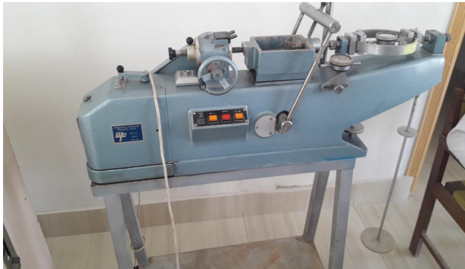
Figure 3.7 Direct Shear Test Apparatus
