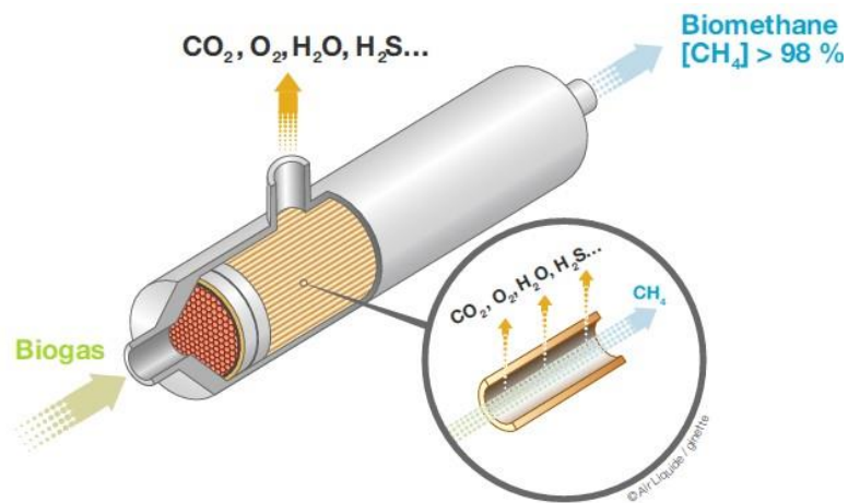
Figure 7: Schematic representation of a Gas Separation Membrane Module
