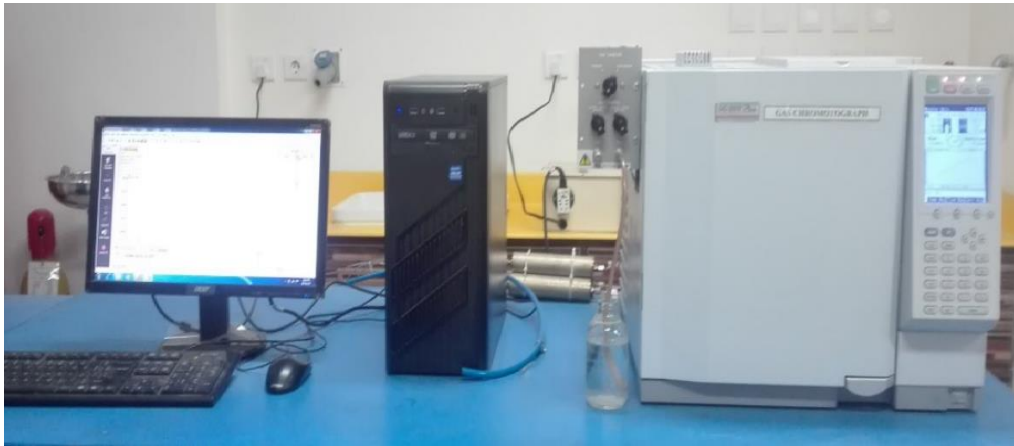
Figure 3.9: SHIMADZU GC-2010 plus gas chromatograph with TCD detector
