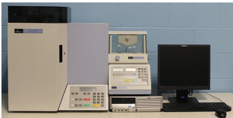
Figure 3.3: CHNS elemental analyzer (PerkinElmer 2400II, USA)
