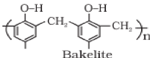
Figure 2.6 Cross linked Structure of Bakelite
