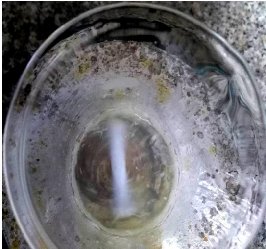
Fig. 2.2. Mixing of precursor and chelating agent
