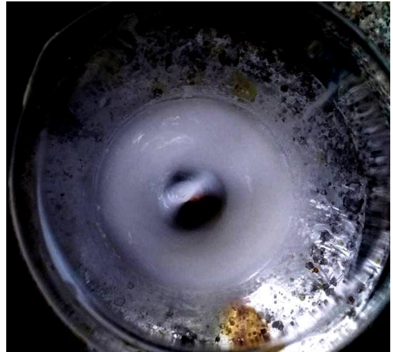
Fig.2.3. Formation of white precipitation upon adding water (hydrolysis)
