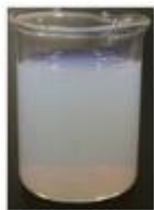
Fig.2.4. Sol-gel after refluxing
