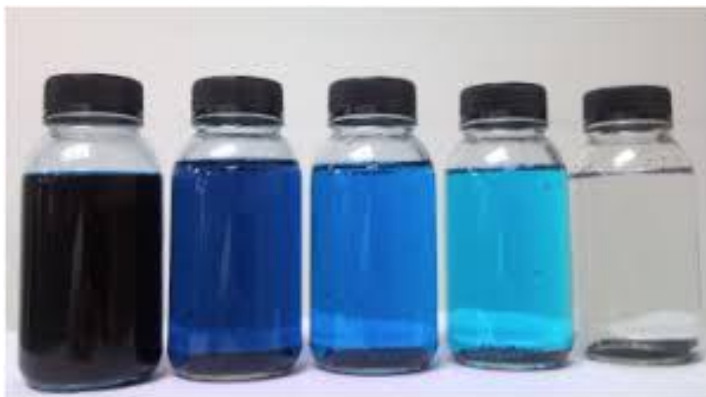
Fig. 4.28. Photocatalytic Degradation of Methylene Blue by Indium doped titania
