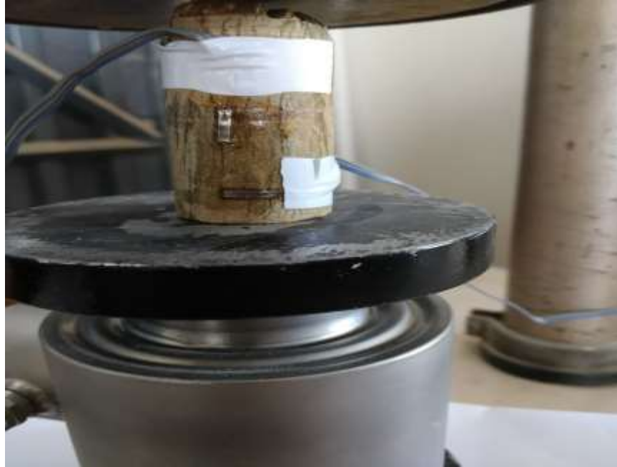
Figure 3-4 Strain gauges on rock core
