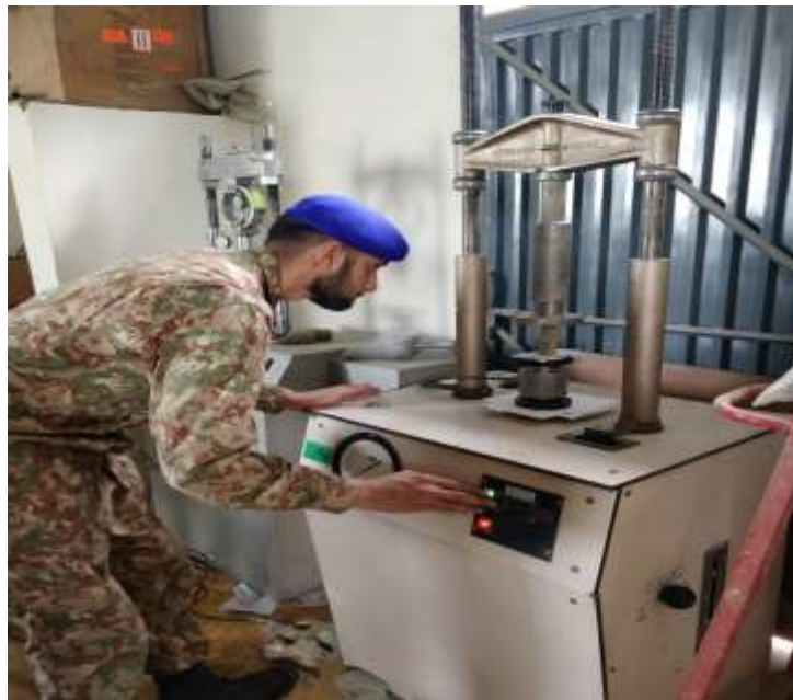
Figure 4-23 Uniaxial compression test
