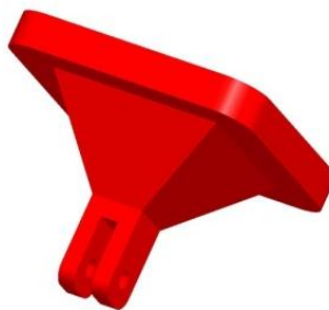
Figure 5.8 : Mechanical Joint between 6 DOF platform Ball screws Actuator
