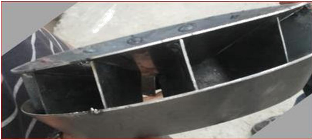
Figure-16 Fabricated Blade profile
