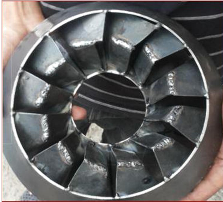
Figure-17 Fabricated blade profile.
