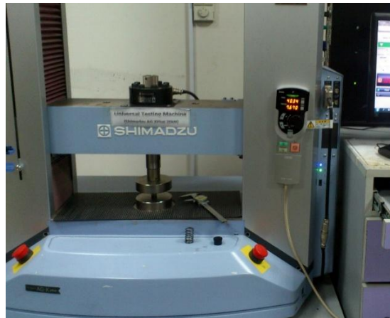
Figure 6: Valve spring testing on Universal Testing Machine (UTM)
