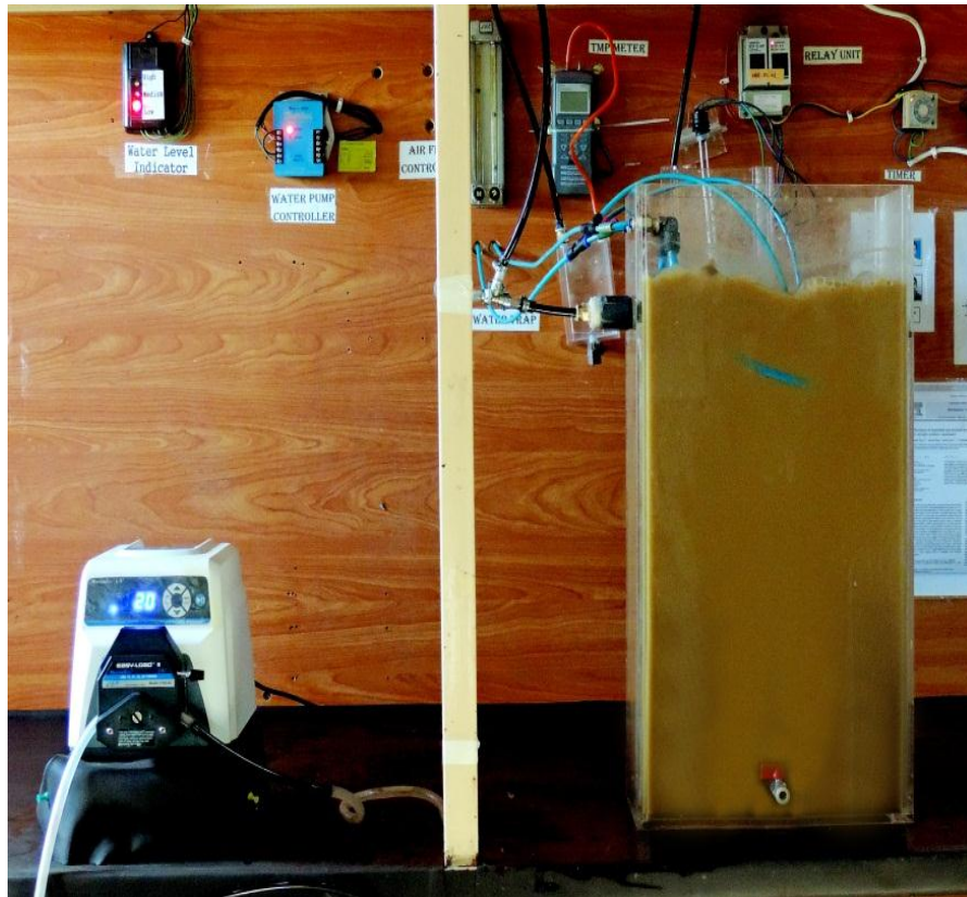
Figure 3.3- Lab scale MBR (a) without sludge (b) with sludge during Phase I
