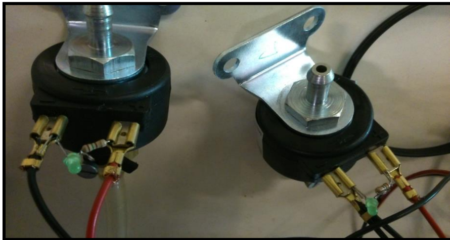
Figure 3.6: Solenoid Valves of the Lab Scale Unit
