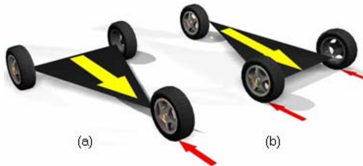
Figure 1-1 Three wheeled Vehicle configurations: a) Delta and b) Tadpole wheel layouts[26]
