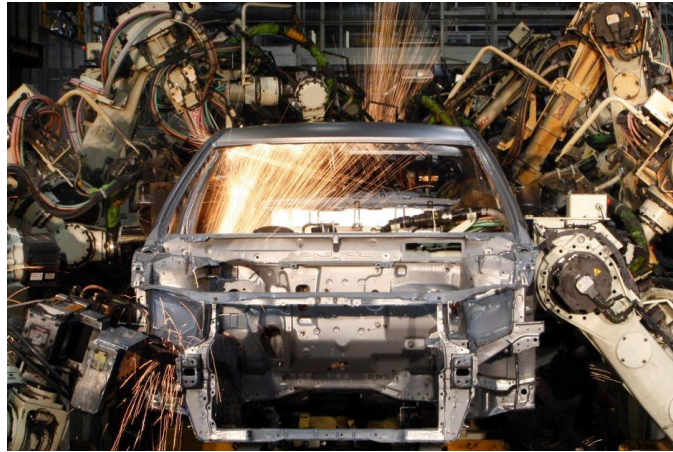
Figure 2: Robot Arm for Welding (Complex Tasks) [2]
