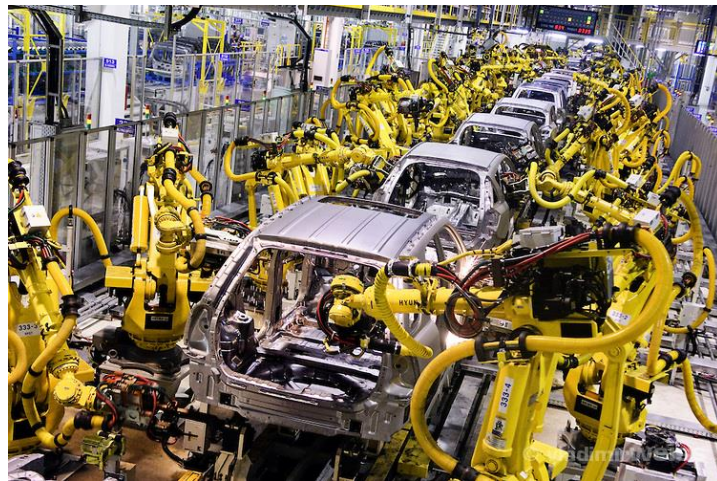
Figure 3: Assembly Line Robots (Repetitive Tasks) [3]
