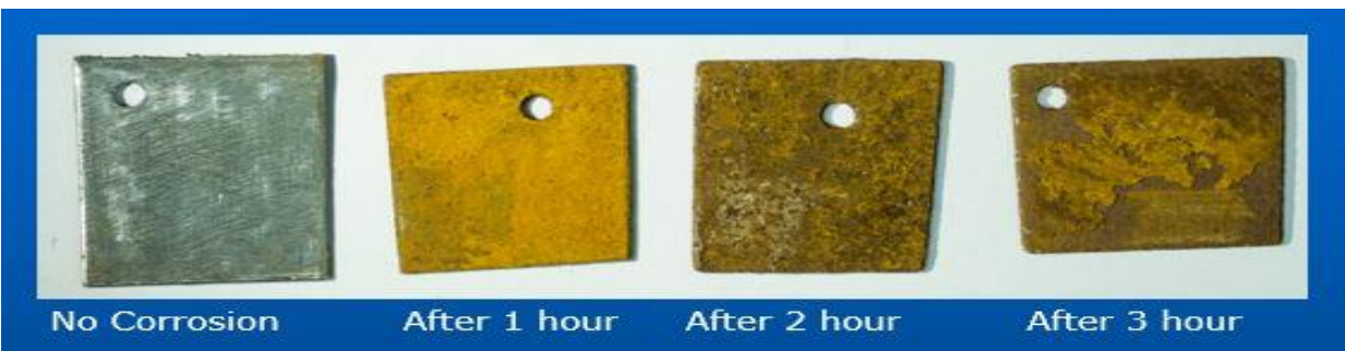
Figure 4. 3: Images of samples after accelerated corrosion testing
