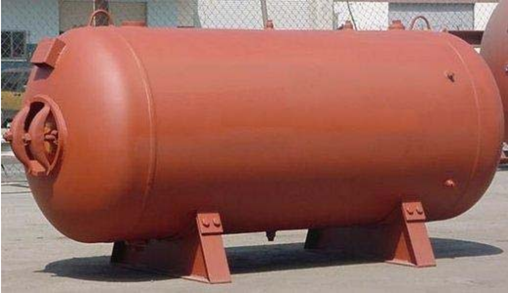
Figure 1.1: A typical pressure vessel
