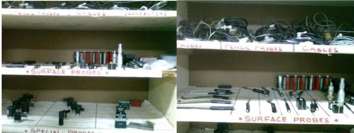
Figure 2-8 Eddy Current Equipment Probes
