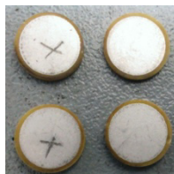
Figure 4-1: PZT-5A equivalent (P33) transducers (unused, + sign indicates positive electrode)
