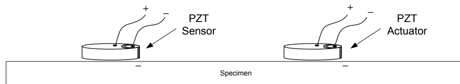
Figure 3-6: Correct electrical alignment for PZT wafers
