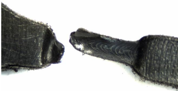
Tensile test @ strain rate 200mm/min
