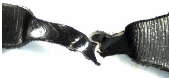
Tensile test @ strain rate 300mm/min
