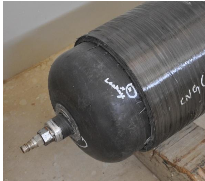
Figure 2.7: Leakage in Type IV CNG Cylinder
