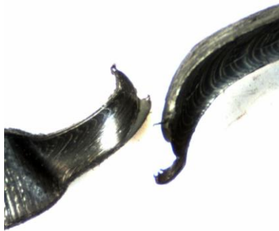
Tensile test @ strain rate 25mm/min
