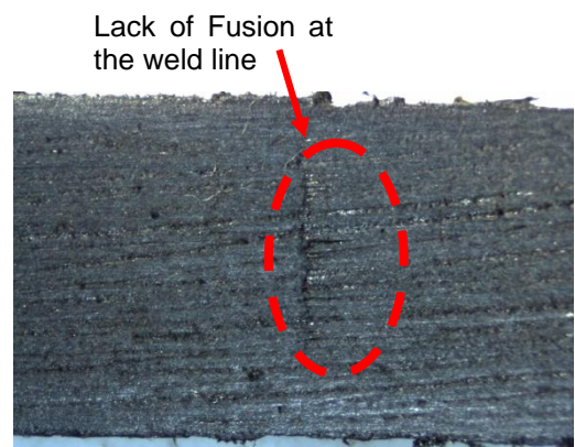
Fusion Joint made @ 200 °C & 3 min (extruded – injection molded)
