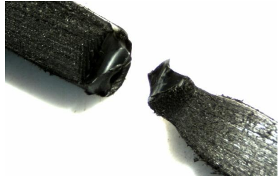
Tensile test @ strain rate 100mm/min
