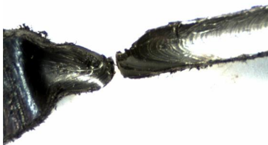
Tensile test @ strain rate 50mm/min
