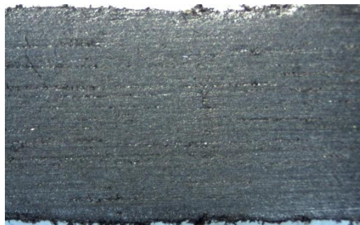
Fusion Joint made @ 250 °C & 3 min (extruded – extruded)
