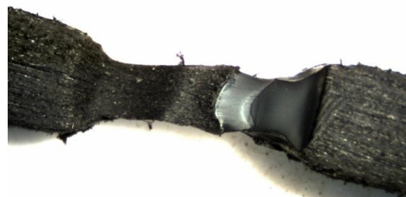
Tensile test @ strain rate 50mm/min
