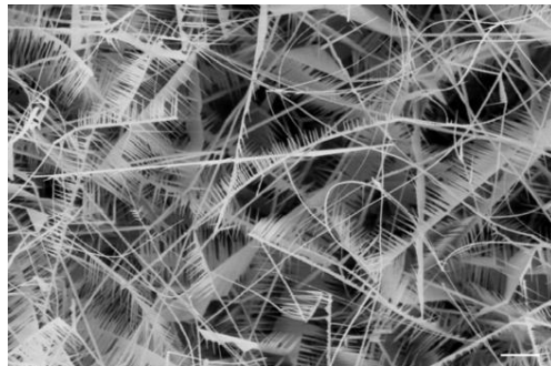
Figure 16 SEM image of nanocombs and saws.[2]
