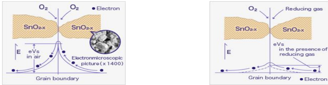
Figure 5: left , absence of reducing gas,and right, presence of reducing gas
