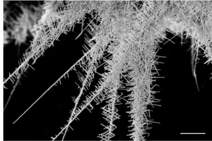
Figure 15 SEM image of the hierarchical ZnO nanostructures.[2]
