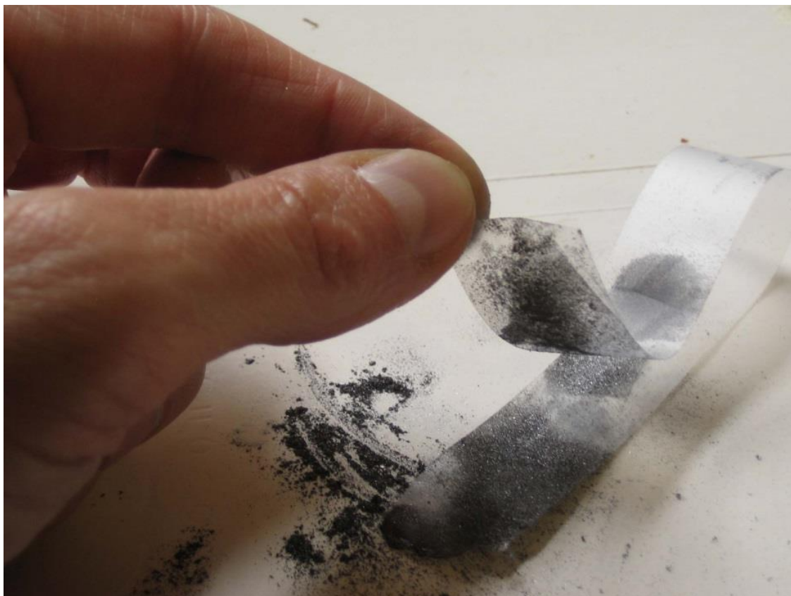
Figure 8: Micromechanical cleavage of graphite to obtain graphene using Scotch tape
