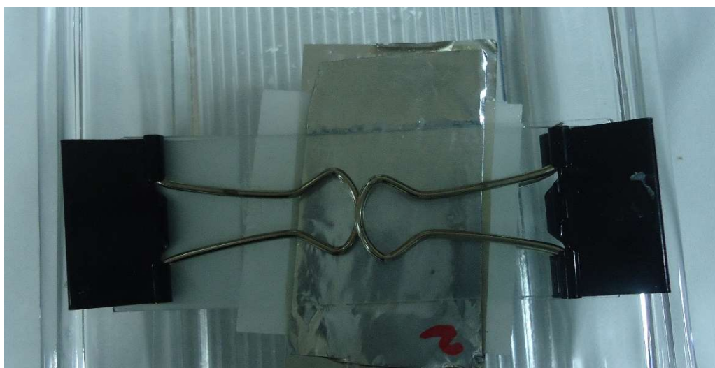
Figure 4.11 Laboratory scale supercapacitor in two electrode configuration
