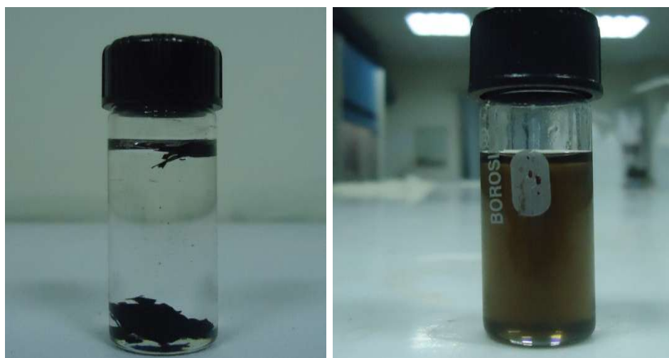
Figure 4.6 (a) GO in DMSO before the sonication (b) GO in DMSO after the sonication in DMSO
