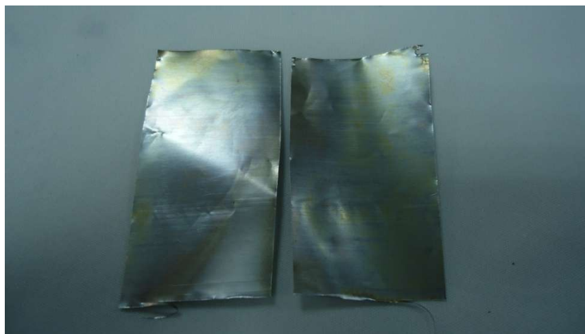
Figure 4.10 Electrodes with f-(LOF)GO drop casted and dried on Al-foil
