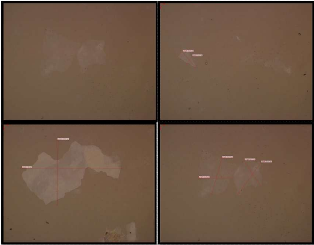
Figure 5.5 Optical images of GO deposited on SiO 2 /Si substrate
