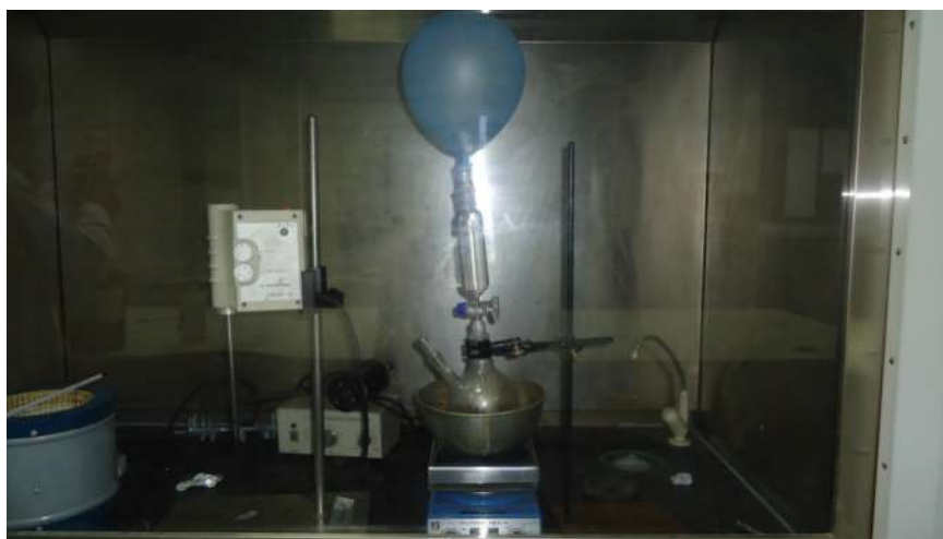
Figure 4.7 Experimental set up for the functionalization of GO
