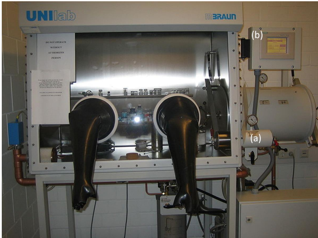
Figure 20: Glove Box (a) Small vacuum chamber (b) Pressure monitoring screen.
