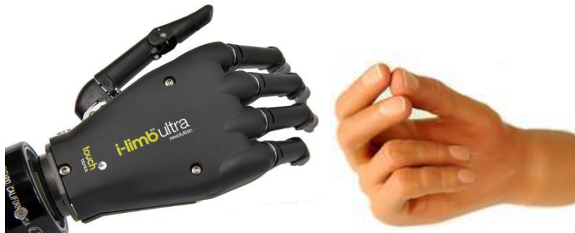
Figure 1.3.1: Anthropomorphic Prosthetic Hands i-LIMB Ultra Revolution & i-LIMB Cosmetic Cover [24]
