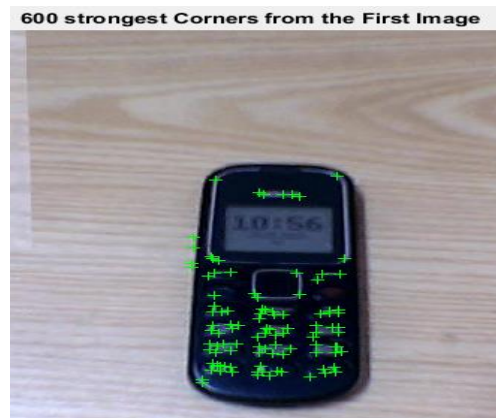
Figure 3.7.4.1.2: Step 01: Selection of 600 SURF Feature Points
