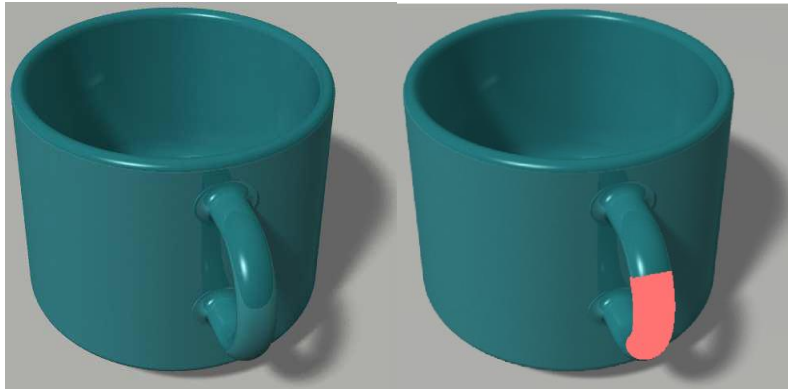
Figure 2.2.5.2.1: The red points in each image show the locations most likely to be a grasping point [24]
