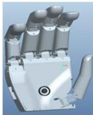
Figure 1.4.1: Pro E model Pro E model of Prosthetic hand with camera embedded in the palm of hand
