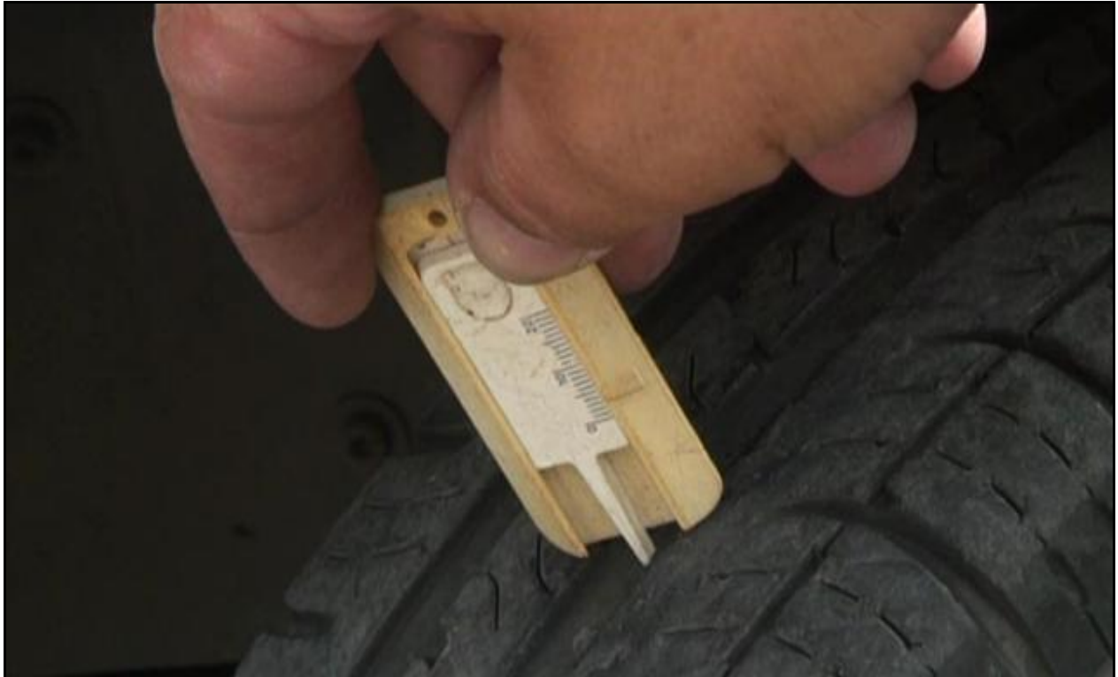
Figure 5.3: Tyre Checking Procedure with Gauge
