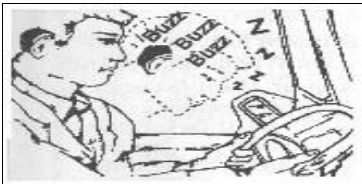
Figure 5.2: Dozing Alert Alarm Mechanism –Buzzing on 15 Degree Head Bend
