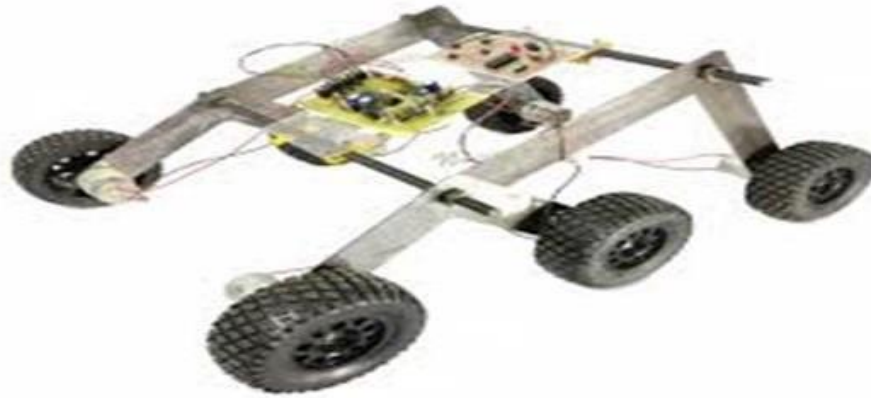
Figure 2.5: Rocker Bogie Mechanism(2)
