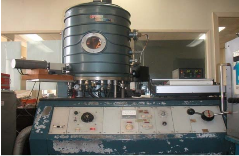
Fig. 3.2: Experimental set up of close spaced sublimation technique at NILOP
