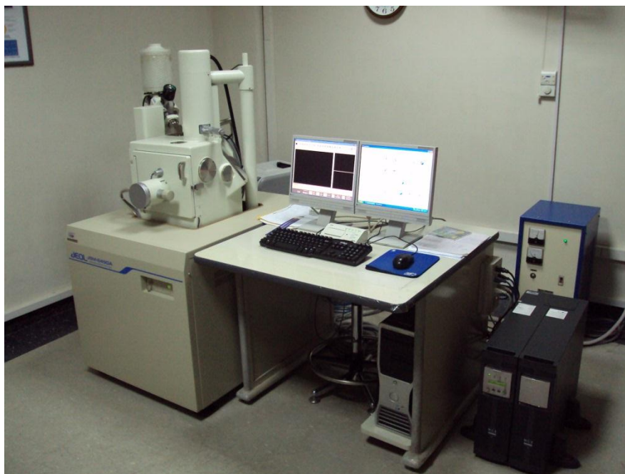
Figure 3.2: JEOL Analytical Scanning Electron Microscope (JEOL JSM-6490A)
