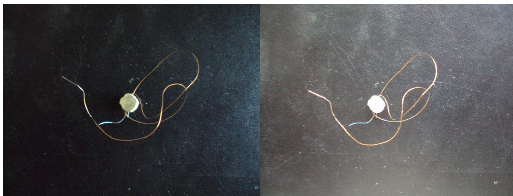
Figure 3.3: BaTiO 3 powder pellet prepared for impedance analysis.
