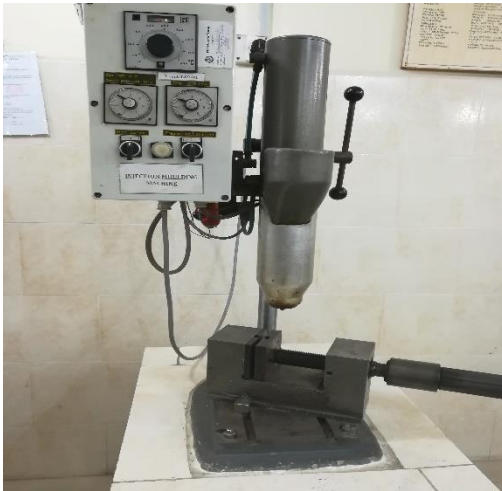
Figure 9 Sample Preparation Unit for Tensile and Impact Sample
