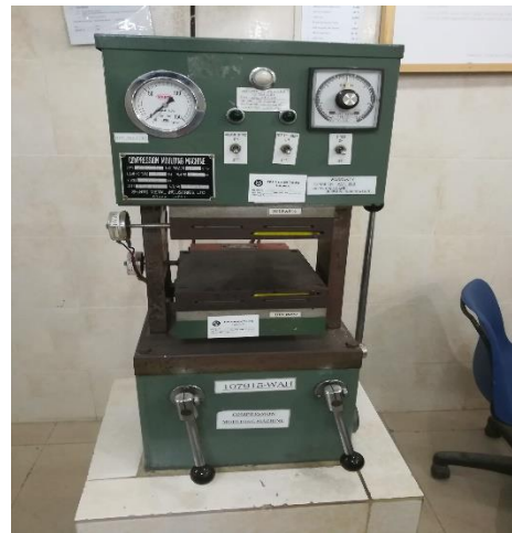
Figure 9 Sample Preparation Unit for Tensile and Impact Sample
