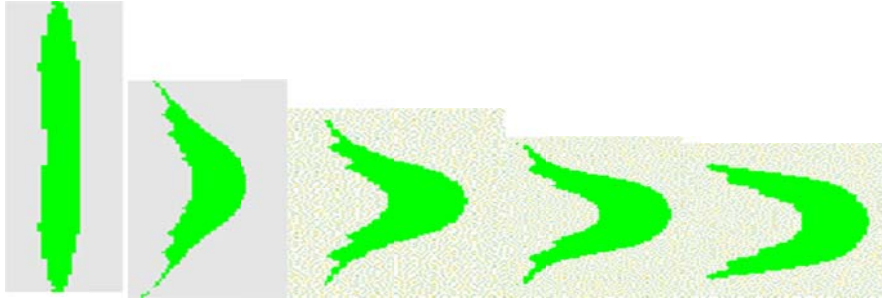
Figure 5.29: formation of Tungsten EFP in void (pictures in zoomed form)(at 20,30,40,50,80 \mu sec)
