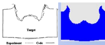
Figure 5.4: Comparison of target penetration cross-section produced by Fe EFP.
