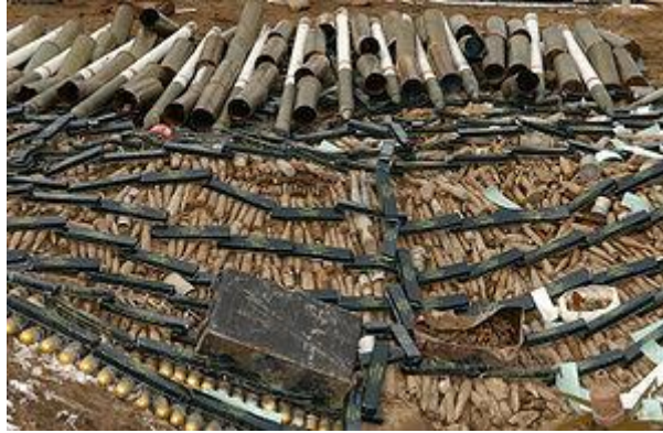
Fig 1.1 1.25-lb M112 demolition charges consisting of a C-4 explosive atop degraded weaponry scheduled for destruction
