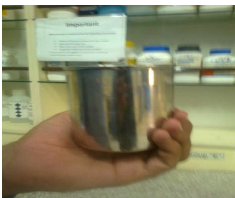
Fig 2.3 Mixing of Acetone & Viton in steel beaker in order to make slurry
