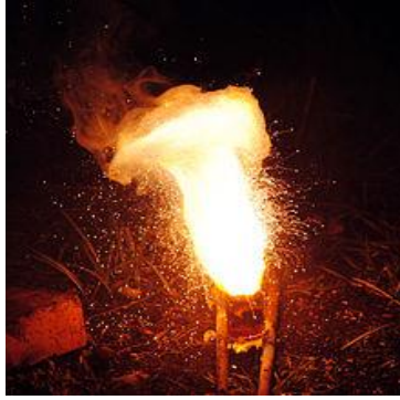
Fig 1.6 A thermite reaction using iron (III) oxide. The sparks flying outwards are globules of molten iron trailing smoke in their wake.
