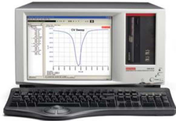
Figure 3. 7: Keithley 4200-SCS for Electrical Characterization [11]
