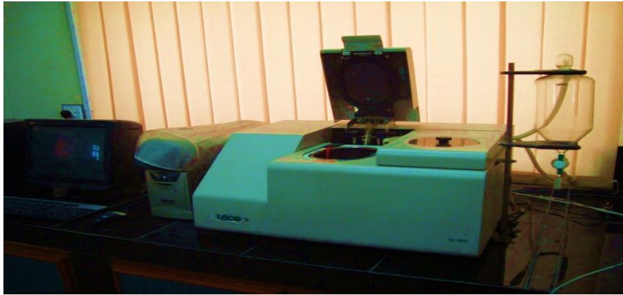
Figure 3.2: Digital Calorimeter (LECO AC-500) in Research lab of Centre for Coal Technology Punjab University Lahore
