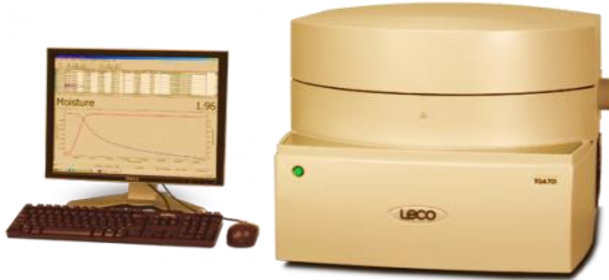
Figure 3.4: TGA 701 leco available in research lab of Centre for coal technology Punjab university
