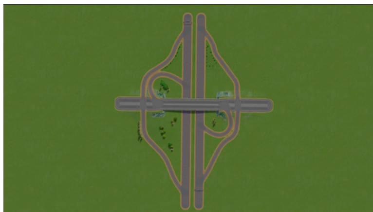
Figure 2.7 Image showing Partial cloverleaf interchange
