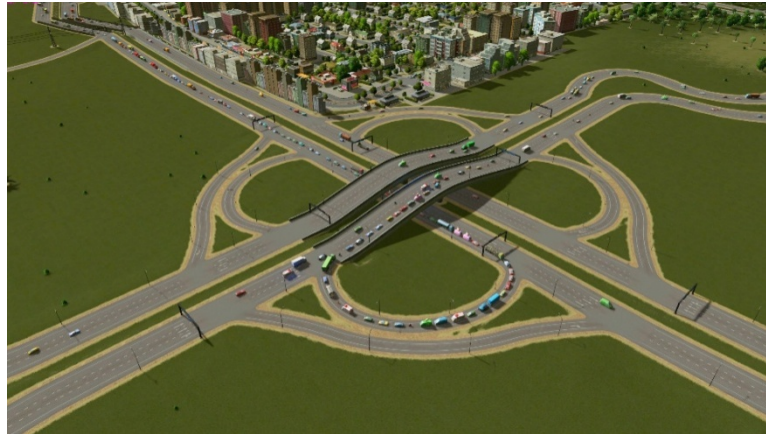
Figure 2.6 Image Showing a Cloverleaf interchange
